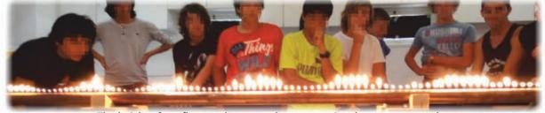
The height of gas flames, show sound waves passing down a copper tube.
